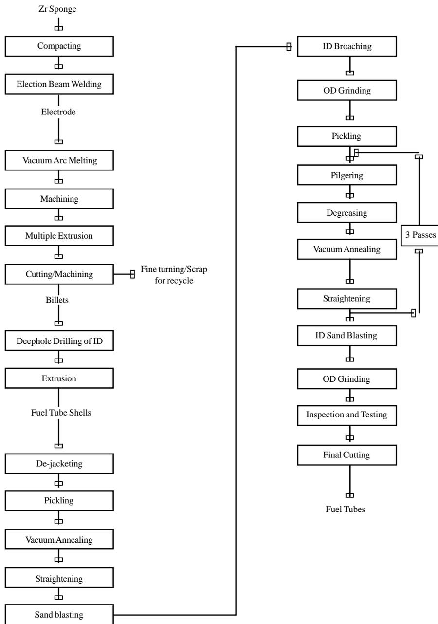
**FIG 7 : PROCESS FLOW SHEET FOR PRODUCTION OF ZIRCALOY FUEL TUBES**
