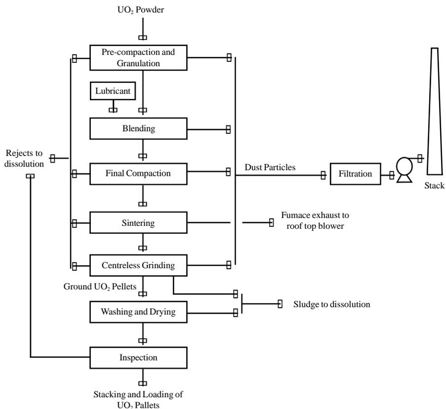
**FIG 3 : PROCESS FLOW SHEET FOR FABRICATION OF  $UO_2$  PELLETS**
