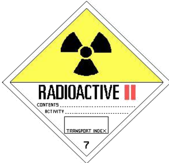
FIG. 3. CATEGORY II-YELLOW LABEL. THE BACKGROUND COLOUR OF THE UPPER HALF OF THE LABEL SHALL BE YELLOW AND THE LOWER HALF WHITE, THE COLOUR OF THE TREFOIL AND THE PRINTING SHALL BE BLACK, AND THE COLOUR OF THE CATEGORY BARS SHALL BE RED.
