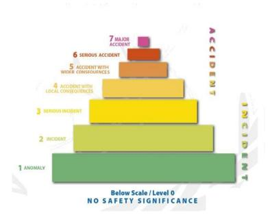
Events rated at level 4 and above are termed as 'Accidents'. The accidents at Chernobyl NPP in former USSR (now in Ukraine) in April 1986 and Fukushima NPPs in Japan in March 2011 were rated at level 7 on INES. Events rated at levels 1, 2 and 3 are called 'Incidents'. Events with no safety significance are rated at level 0 or below scale.
