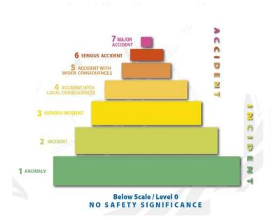
Events rated at level 4 and above are termed as 'Accidents'. The accidents at Chernobyl NPP in former USSR (now in Ukraine) in April 1986 and Fukushima NPPs in Japan in March 2011 were rated at level 7 on INES. Events rated at levels 1, 2 and 3 are called 'Incidents'. Events with no safety significance are rated at level 0 or below scale.
