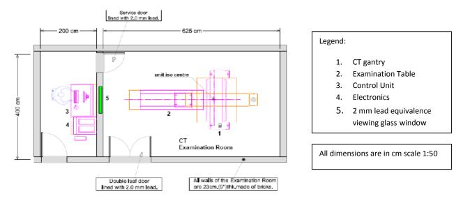
\*Note: Same type of room layout plan can be used for testing of Cath Lab equipment.
