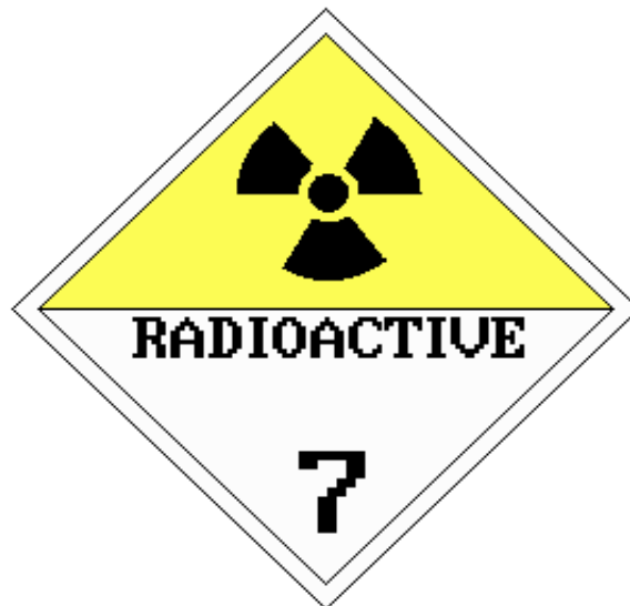
FIG. 6. PLACARD. EXCEPT AS PERMITTED BY CLAUSE 6.15.4.1, MINIMUM DIMENSIONS SHALL BE AS SHOWN; WHEN DIFFERENT DIMENSIONS ARE USED, THE RELATIVE PROPORTIONS SHALL BE MAINTAINED. THE NUMBER '7' SHALL NOT BE LESS THAN 25 mm HIGH. THE BACKGROUND COLOUR OF THE UPPER HALF OF THE PLACARD SHALL BE YELLOW AND THE LOWER HALF WHITE, THE COLOUR OF THE TREFOIL AND THE PRINTING SHALL BE BLACK. THE USE OF THE WORD 'RADIOACTIVE' IN THE BOTTOM HALF IS OPTIONAL, TO ALLOW THE ALTERNATIVE USE OF THIS PLACARD TO DISPLAY THE APPROPRIATE UN NUMBER FOR THE CONSIGNMENT.
