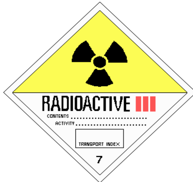
FIG. 4. CATEGORY III-YELLOW LABEL. THE BACKGROUND COLOUR OF THE UPPER HALF OF THE LABEL SHALL BE YELLOW AND THE LOWER HALF WHITE, THE COLOUR OF THE TREFOIL AND THE PRINTING SHALL BE BLACK, AND THE COLOUR OF THE CATEGORY BARS SHALL BE RED.
