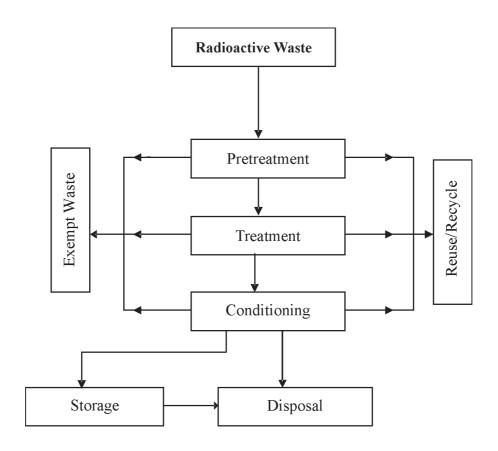
FIG. A-1: BASIC STEPS IN RADIOACTIVE WASTE MANAGEMENT
