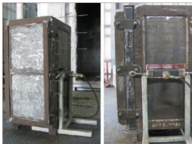
Figure 7.8.1 (a): Reduced Scale Facility for Testing FR Panels
