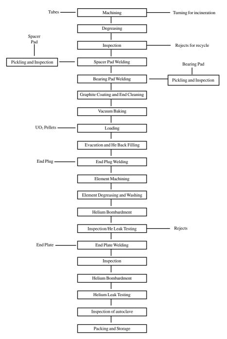
FIG 4 : PROCESS FLOW SHEET FOR FUEL ASSEMBLY
